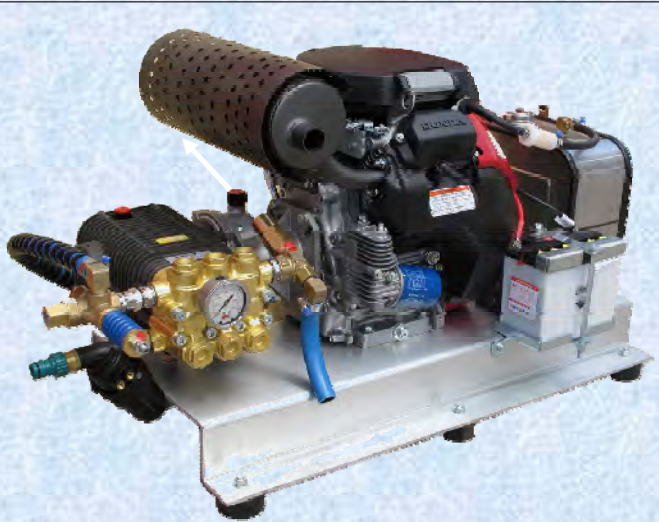
BAR2727G-HEB Gear Box Drive 2500 Psi 42 l/min. Gear Box Drive, Electric Start on Base Plate Honda 27Hp, Comet TW11025 Pump Gear Box Drive Trade Price $6,999
