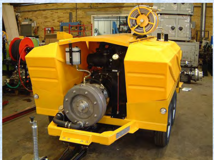
Harben 4020-Hi Q 4000Psi / 90 l/min. Suitable for Plumbing Contracting or Industrial Cleaning Isuzu or Perkins 80Hp Diesel, Harben P Pump Supplied complete with a registered trailer - Twin water Tanks Trade Price $82,500
