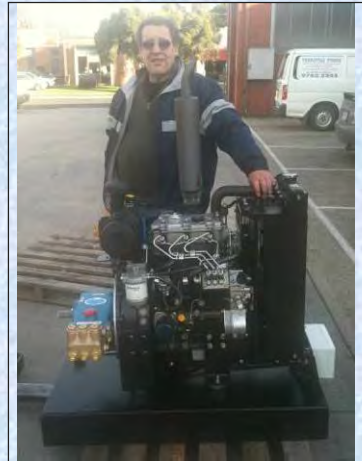
BAR3030P-PS 3000 Psi 30 l/min. Perkins Water Cooled 30Hp on Skid CAT 660 Pump Trade Price $24,999
