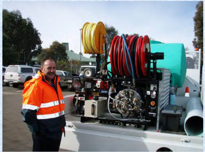
Harben 3516-Van Pack 3500Psi / 70 l/min. Delivered to Central Highlands Water Yanmar TNV88 42Hp Diesel, Harben P Pump Supplied as van Pack..fitted to customers truck Trade Price $53,900
