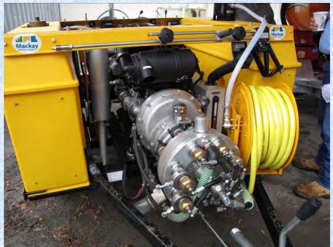
Harben 3516-DTB 3500Psi / 70 l/min. Delivered to Mackay Municipal Council Yanmar 40Hp Diesel, Harben P Pump Supplied complete with a registered trailer - Twin water Tanks Trade Price $53,900
