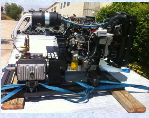
BAR7238G-KEB 7250Psi 38 l/min. Kohler 2204T 4 Cylinder Water Cooled Turbo Diesel HPP Pemium Pump Drive - Belt Drive Skid Mounted Trade Price $poa
